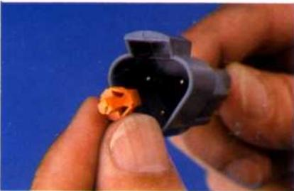
4 Once all contacts are in place, insert orange wedge with arrow pointing toward exterior locking mechanism. The orange wedge will snap into place. Rectangular wedges are not oriented. They may go in either way.
