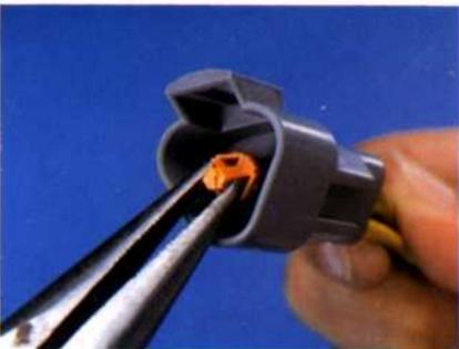
1 Remove orange wedge using needlenose pliers or a hook shaped wire to pull wedge straight out.
