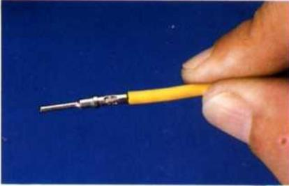
1 Grasp crimped contact approximately (25.4 mm) one inch behind the contact barrel.
