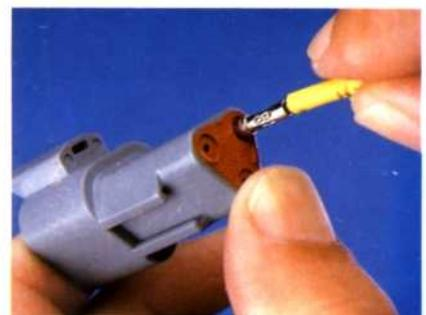
3 Hold the rear seal in place, as removing the contact will displace the seal.
