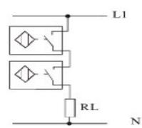
◆Parallel connection of two-wire AC sensor
