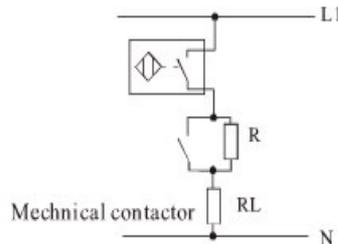
◆ Parallel connection of machinery switch and AC sensor
