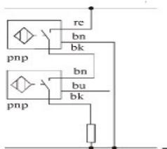
◆Parallel connection of three-wire DC and three-wire DC sensor
