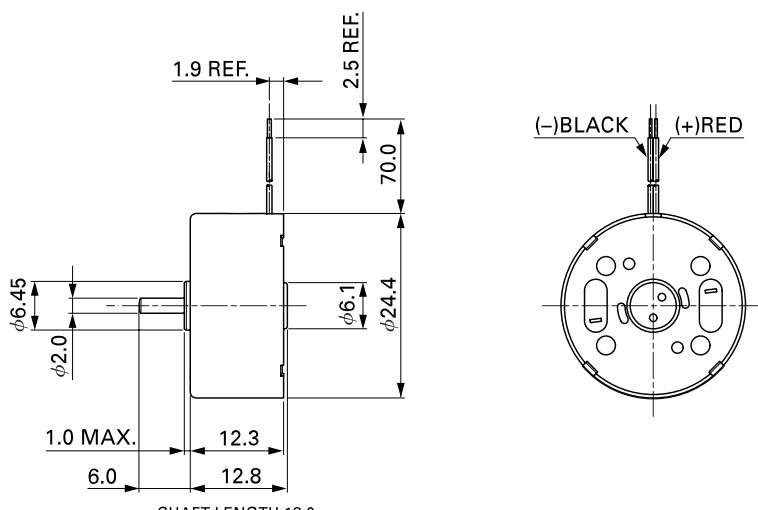
Usable machine screw length 1.1 max. from motor mounting surface.
